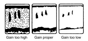
Figure 2-17 Examples of proper and improper gain
